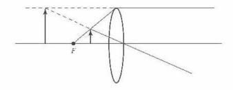
**34.24:** a)  $\frac{1}{s} + \frac{1}{s'} = \frac{1}{f} \Rightarrow \frac{1}{f} = \frac{1}{16.0 \text{ cm}} + \frac{1}{-12.0 \text{ cm}} \Rightarrow f = -48.0 \text{ cm}, \text{ and the lens is}$
